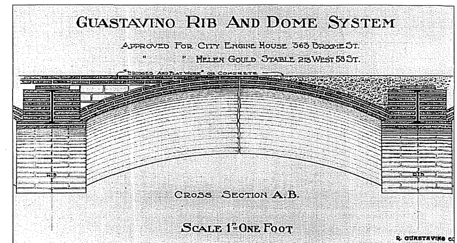
Guastavino Rib and Dome System, Gould Stable and City Engine House at Broome Street, New York, 1902 (FROM J. PARKS AND A. NEUMANN, THE OLD WORLD BUILDS THE NEW (AVERY LIBRARY, 1996))
